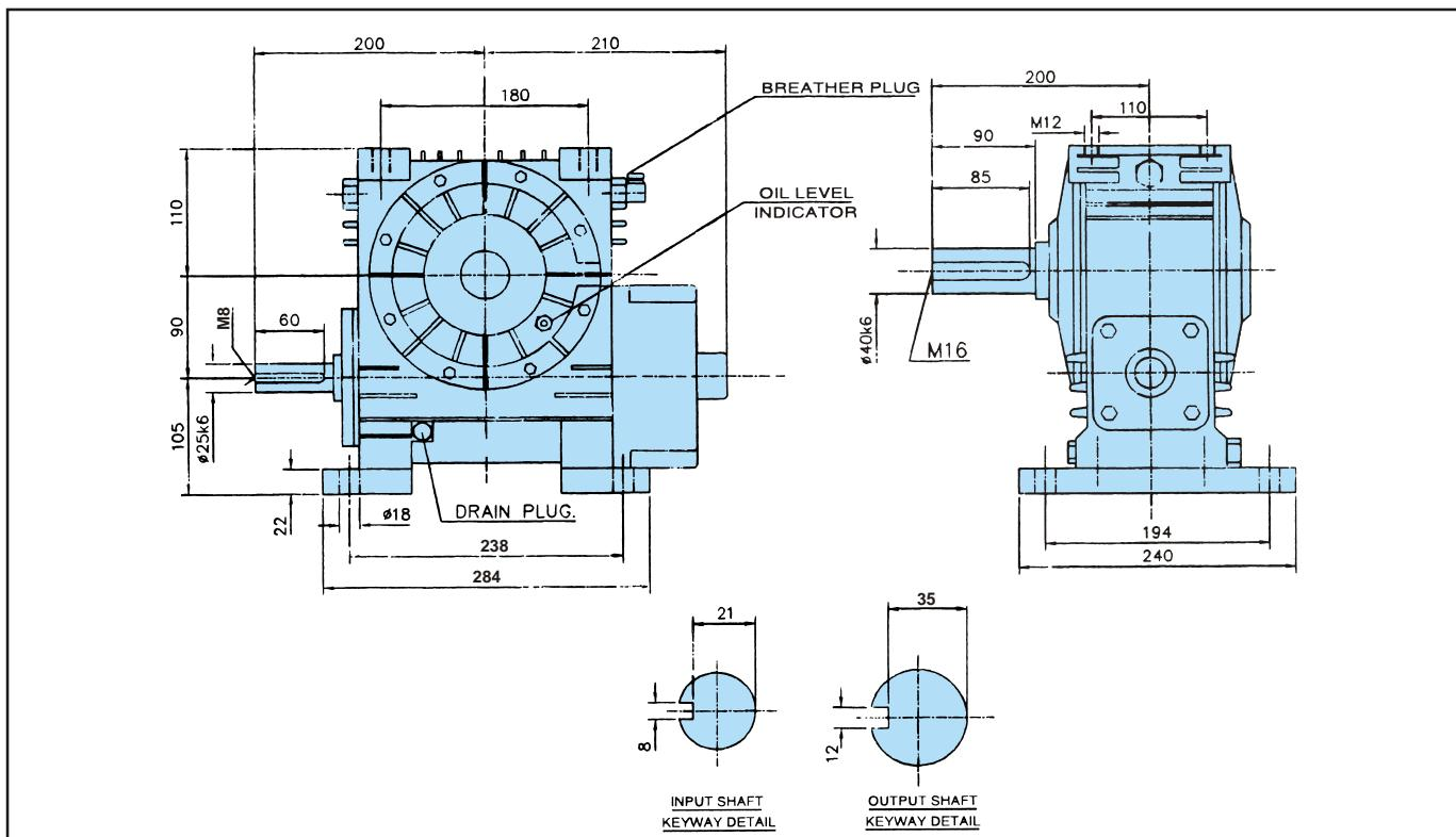
Key & Keyways as per IS 2048. Shaft limits up to 58dia.-k6 and above 58 dia.-m6
