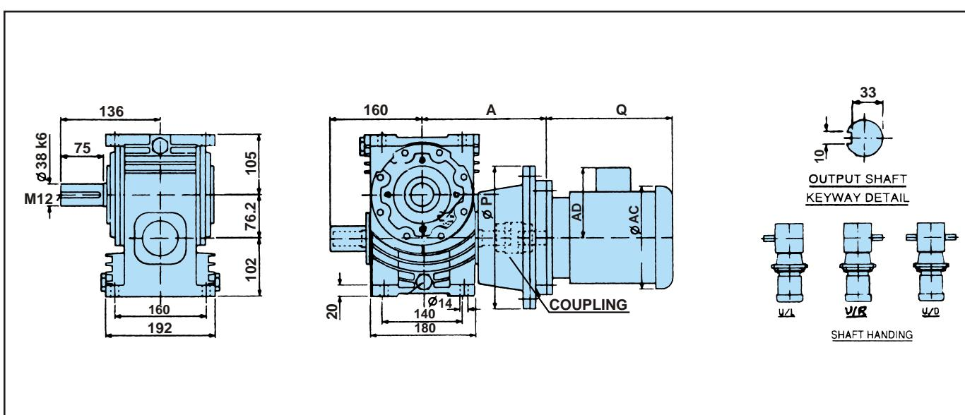
Key & Keyways as per IS 2048. Shaft limits upto 58dia.-k6 and above 58 dia.-m6
