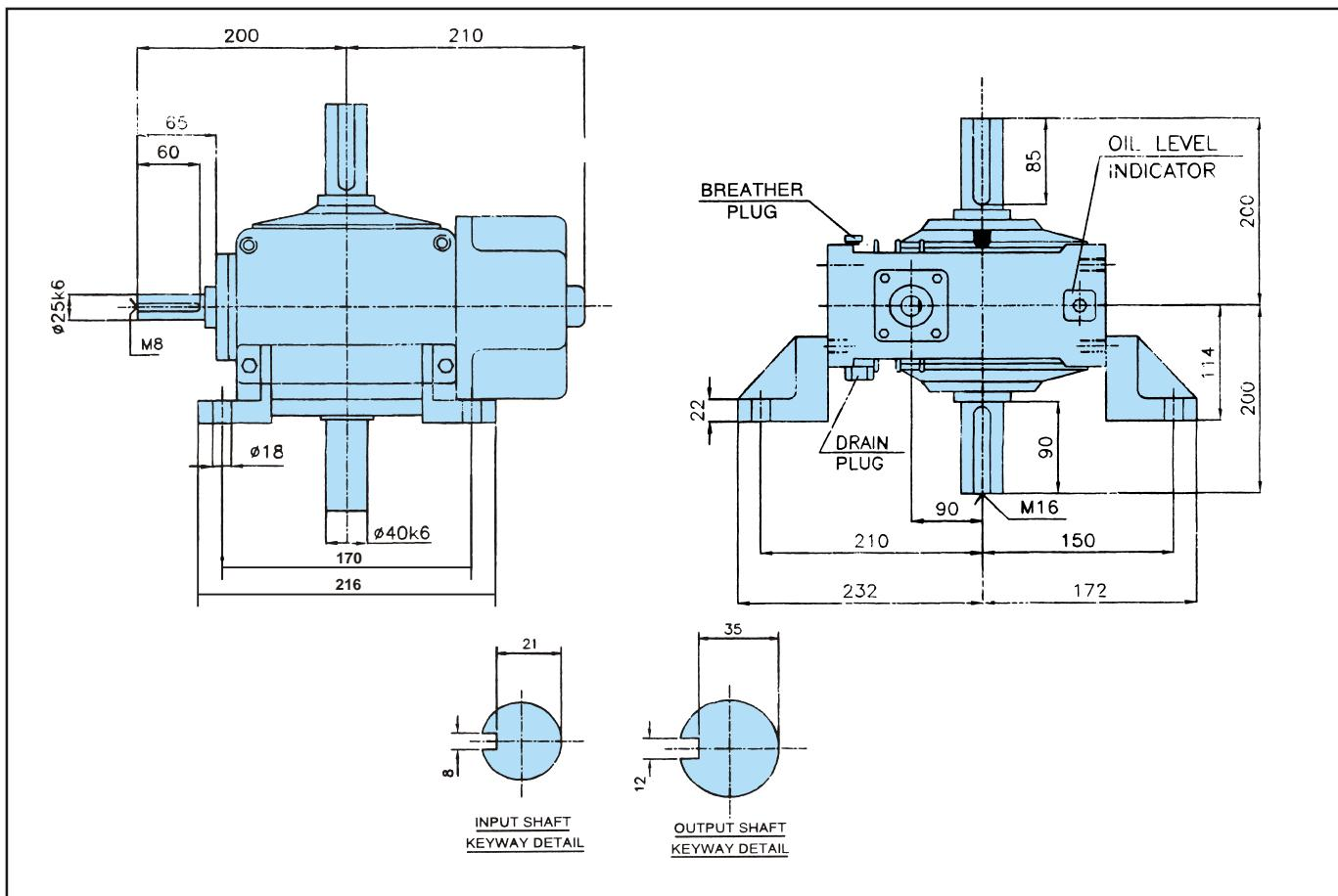
Key & Keyways as per IS 2048. Shaft limits up to 58dia.-k6 and above 58 dia.-m6
