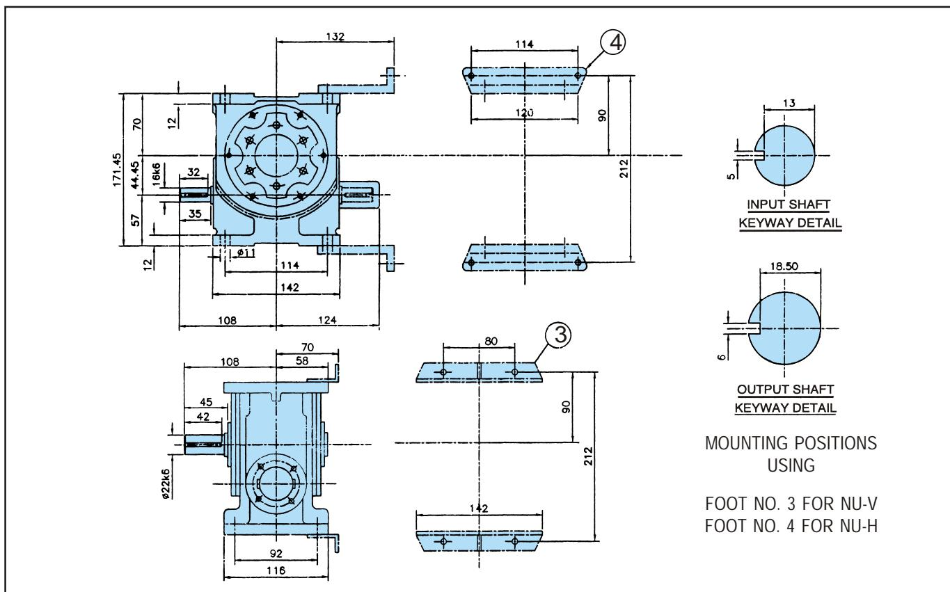
Key & Keyways as per IS 2048. Shaft limits up to 58dia.-k6 and above 58 dia.-m6
